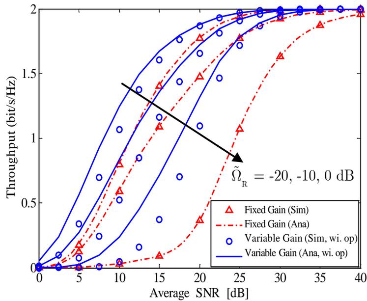
Fig. 6. The system throughput of the variable gain FD relaying system versus the average SNR at the relay node for the case using optimal power allocation and different RSIs,  $\mathcal{R} = 2$ ,  $\Omega_3 = 0.01$ .
