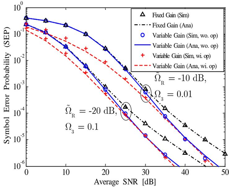
Fig. 8. The SEP of the considered fixed/variable gain FD relaying system versus the average SNR  $= P_S/\sigma_R^2$  for different channel gains and RSIs. The transmission power of the relay node is fixed so that  $P_R/\sigma_D^2 = 25$  dB.
