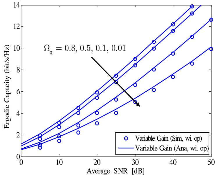
Fig. 9. The ergodic capacity of the variable gain relaying system versus the average SNR at the relay node using optimal power allocation,  $\bar{\Omega}_R = -10$  dB.
